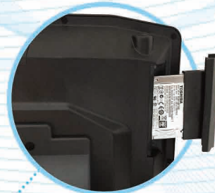
Removable HDD/SSD Easy Maintenance
