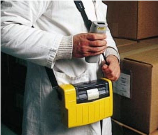
Wireless infrared communication via integrated IrDA port
