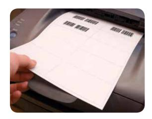
Laser printers can be used to print a large variety of media, from plain paper to specialty papers to films and transparencies. However, when printing on anything other than plain paper, special precautions must be taken, such as the use of laser-specific media, custom printer components, and special maintenance procedures. These special precautions must also be taken to print labels reliably because of the way the laser printer is designed.
