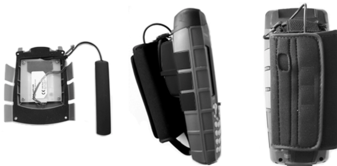
tt8000 with black BackPack and ext. UHF antenna in the big hand strap
