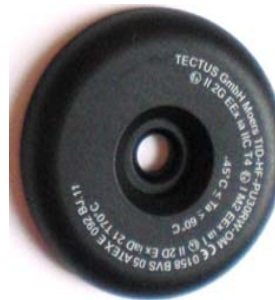
6 mm / 18 mm and 32 mm ATEX TAG TID-UHF-MTP6 / 17 / 32RW
