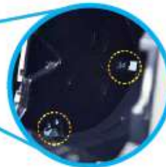
Two paper near end sensors for different direction paper feeding
