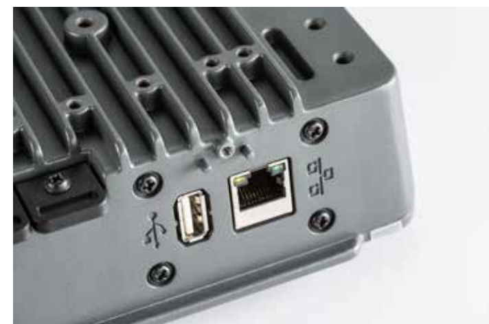
Ethernet RJ45 USB Host type A (USB for software upgrades only)
