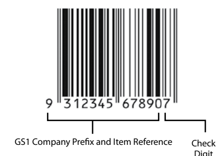
Example of a GTIN-13 represented in an EAN-13 Bar Code
