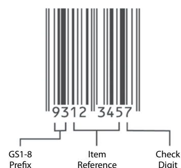
Example of a GTIN-8 represented in an EAN-8 Bar Code
