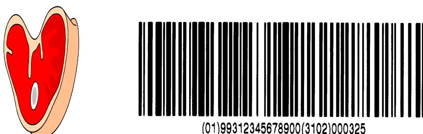
Figure 23: Variable Measure Trade Item with a weight of 3.25kg represented in a GS1-128 Bar Code
