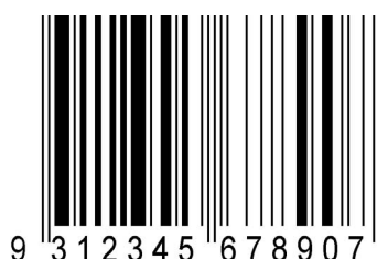
Figure 12: Example of an EAN-13 Bar Code representing the GTIN-13
