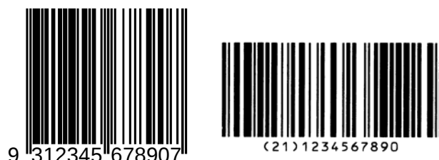
Figure 4: GTIN with attribute information in separate bar codes. GTIN-13 represented in an EAN-13 Bar Code, along side a serial number represented in a GS1-128 Bar Code.
