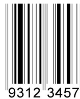
Figure 14: Example of an EAN-8 Bar Code representing the GTIN-8
